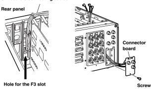
7 Connect the connecting cables to the SDTI board.
