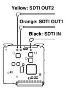
**8** Reinsert the SDI board in the F3 slot, then insert the SDTI board in the same F3 slot located on the front panel side.
