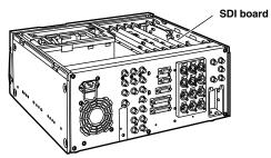
Attach the accessory connector board to the rear panel. As shown in the diagram below, after passing the SDI board's connecting cables through the hole provided for the F3 slot, plug them into the top section of the connector board and then fix the connector board in place using the screw.
